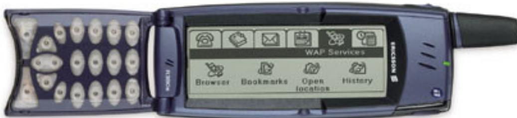
Freshly baked from the oven, the OS underneath Ericsson R380 was actually EPOC Release 5 Unicode or ER5.1 which in one way or another, was the same OS which powered Psion ER5 devices (eg netBook, 5mx etc). The difference between Psion devices and the R380 was in the UI (User Interface). While Psions are using what is famously known as EIKON, the R380 used a new UI developed by Ericsson called ECK (Ericsson Component Kit). Almost 95% of the OS are identical to the one underneath Psion machines.
